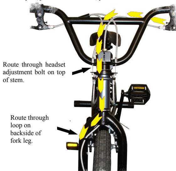
Cable routing diagram for front calliper brake
